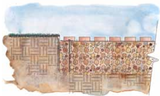
Compacted sandy gravel road base placed above compacted subgrade, 95% modified Proctor density. Gravelpave 2 rolls are laid, pinned, and filled with clean, sharp gravel.
