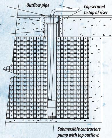
Sections of Rainstore<sup>3</sup> structure that must be removed to allow space for PVC riser. Separate plastic connections with utility knife or heavy shears.
